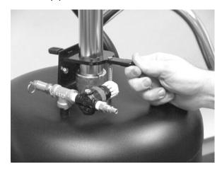
When the bowl is at the desired position, release the locking bar to secure the bowl and drain pipe in place.
