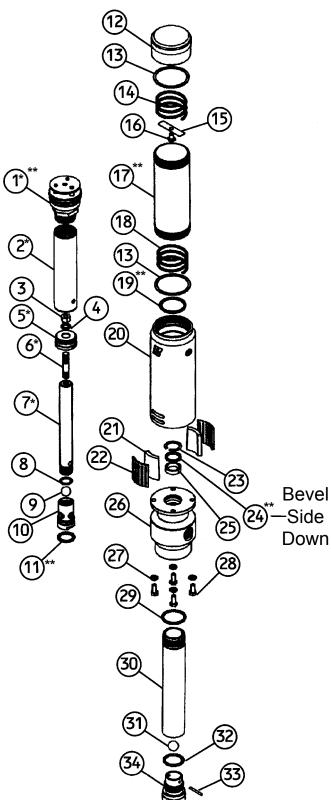
\*Apply Red Loctite (271) on threads where indicated.
