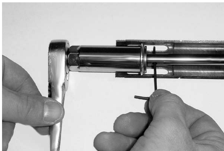
Fig. 1: Removing Grease Intake Assembly
