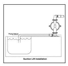
In **suction lift installations** the pump datum is above the fluid line. IMPORTANT: each pump has different lift capabilities. Be sure to verify the lift capability of a particular pump before installing it into a system.
