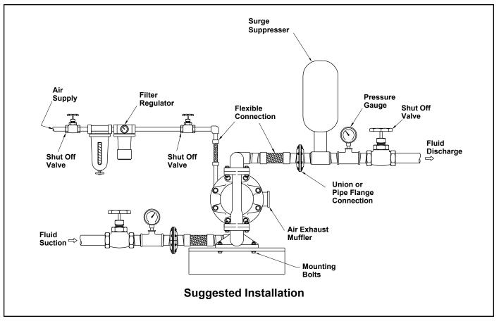
A typical installation showing all the components that are recommended in a system, including valves, pressure gauges, air regulators, filters, and surge suppressors.
