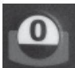
Alphanumeric Keys: Used to enter numbers and alpha characters. Press and release the desired key to enter a number. To enter a letter, press and hold the key with the desired letter. When the desired letter displays, release the key.
