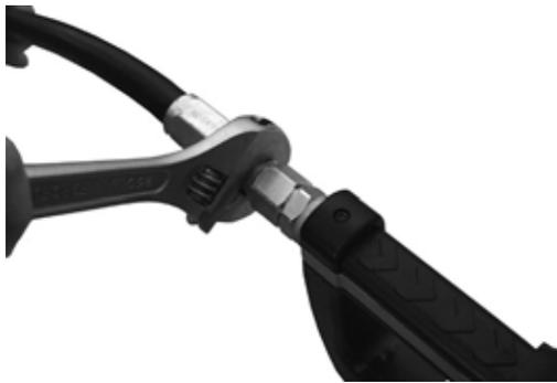
2. Insert the metal end of the hose into the swivel. Tighten completely with an open ended, adjustable, wrench.
