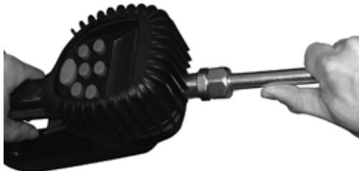
1. On the opposite end, apply sealant to the end of the nozzle. Recommended sealant is Loctite® 243.
