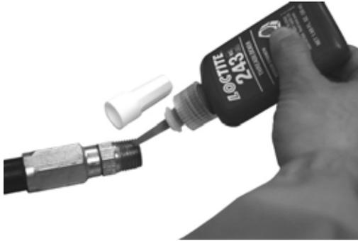
1. Attach a swivel to the meter. Apply thread sealant to the male end of hose. Recommended sealant is Loctite® 243.
