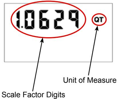
1. Press the **RESET** button to advance through the Scale Factor digits.
