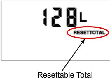
1. Press and hold the **TOTAL** button to see the Accumulated Total.
