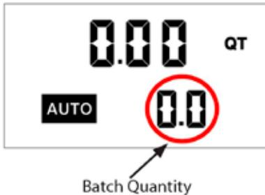
To enter the Batch Mode from the Manual Mode, press the **AUTO** button.
