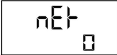
The Radio Network is used to differentiate multiple FMS networks. For standard installations the default setting of zero will not need to be changed.
