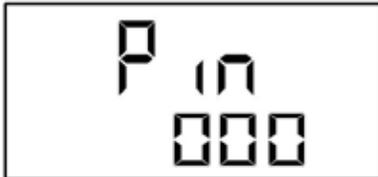
Push the **AUTO** and **TOTAL** buttons at the same time and hold for 2 seconds to bring up the *Program PIN* screen. (**Installers should contact Balcrank to obtain the Programming PIN**), to enter the PIN:
