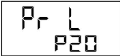
1. The radio power level is set at the factory. The display is for validation purposes only.
