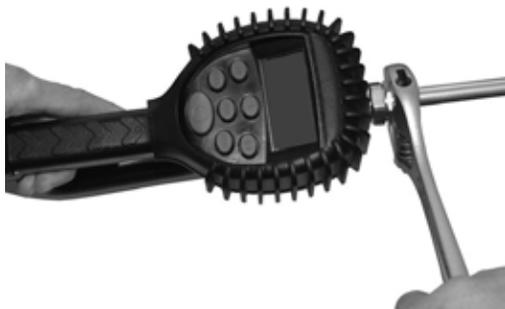
2. Thread the nozzle onto the meter. Screw it in tightly with an open ended, adjustable, wrench.
