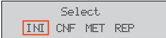
The *INI* menu can be accessed only when the Dispense Order (WO) list is empty. The supervisor must clear all transactions through *Configure (CNF)* before the INI menu becomes available. Refer to “CONFIGURATION (CNF) MENU” on page 15 for details on clearing transactions.
