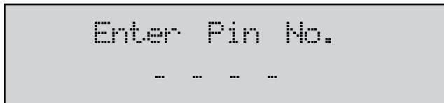
The second default screen is used by the supervisor to access the management screens: Initialization, Configuration, Meter, Report (External Printer), 190 (Internal Printer) and Radio. There can be only one supervisor account per keypad.
