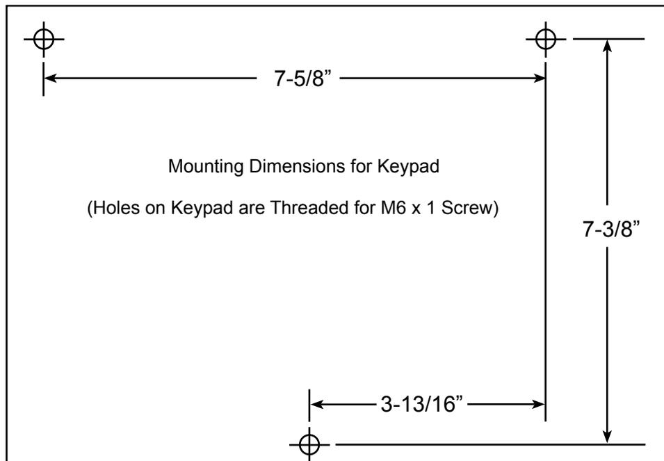
Figure 1: Keypad Installation
