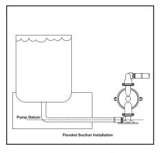
A flooded suction installation has the pump datum line below the fluid level. IMPORTANT: in flooded suction installations the pressure at the fluid inlet of the pump should never exceed 69 kPa (10 psi).
