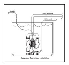
In a **submerged application**, the air exhaust port of the pump must be ported above the fluid line. Be certain that the fluid being pumped is compatible with the materials on both the airside and the wetted side of the pump before the pump is submerged.
