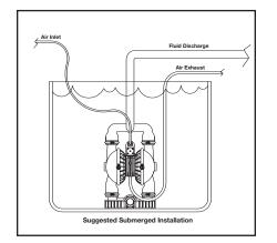
In a **submerged application**, the air exhaust port of the pump must be ported above the fluid line. Be certain that the fluid being pumped is compatible with the materials on both the airside and the wetted side of the pump before the pump is submerged.
