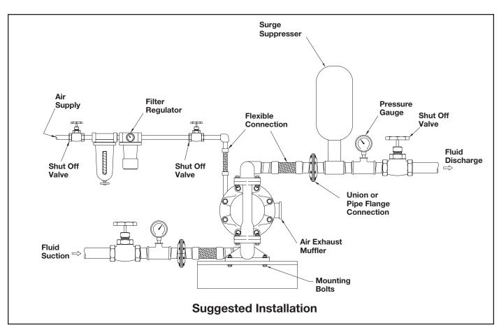
A typical installation showing all the components that are recommended in a system, including valves, pressure
