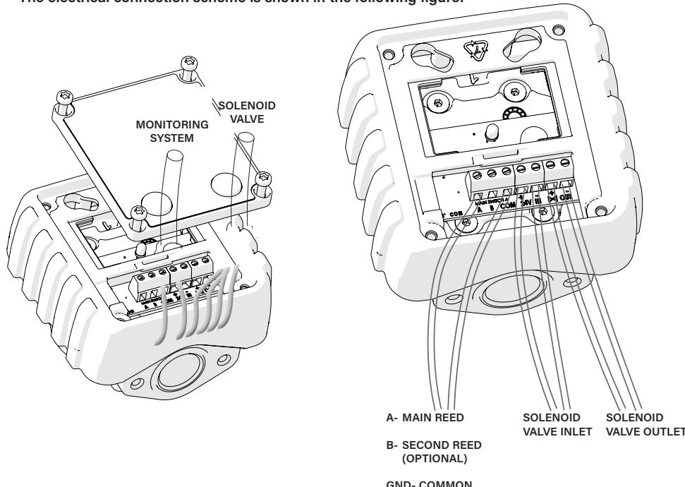
The electronic board LED allows quick display of the open (LED on) or closed (LED off) state of the solenoid valve, if that is installed on the line. Ensure proper connection to the positive and negative poles of the electronic board. The power supply unit must not exceed 30 VDC. The monitoring system responsible for processing the pulses generated will be connected to terminals A, COM and B as follows:
