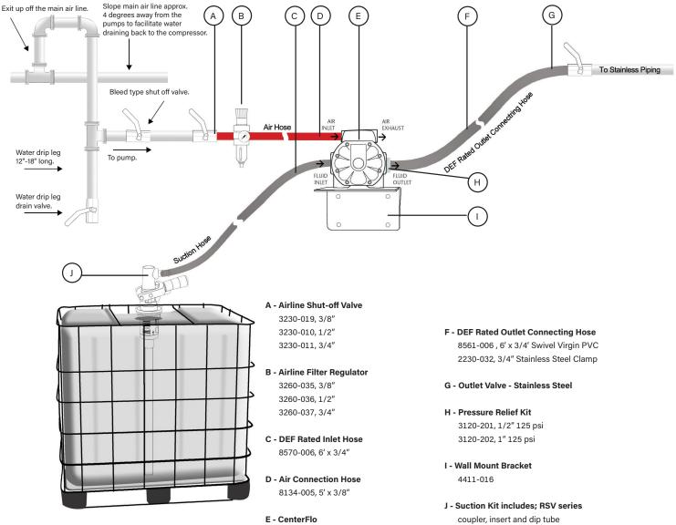
1120-025A, CF15 Poly/BSPP AODD 1120-031A, CF30 Poly/BSPP AODD - Suction Kit includes; RSV serie coupler, insert and dip tube 4530-045, 275 gal tote 4530-046, 330 gal
