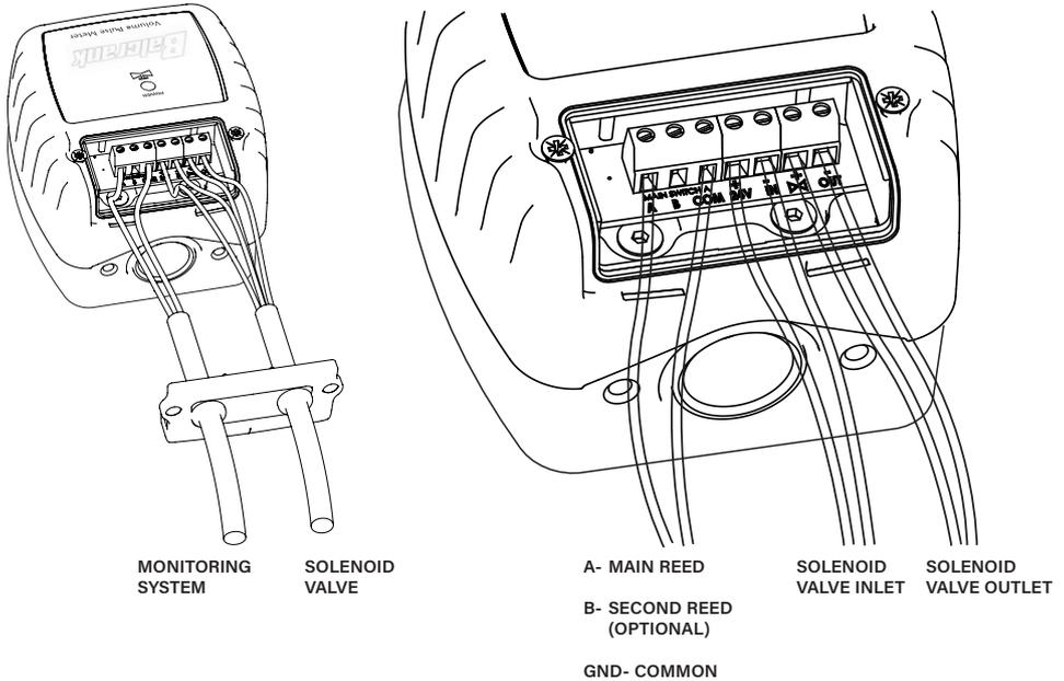
The electronic board LED allows quick display of the open (LED on) or closed (LED off) state of the solenoid valve, if that is installed on the line.
