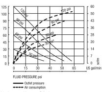
(\*) 2 bar test with a Hytrel\* diaphragms pump.
